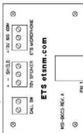
CONNECTIONS TO MSI-BOC5 (SEPARATE MICROPHONE AND SPEAKER)
