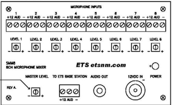
TO AUDIO "LINE IN" OF DVR, I/P CAMERA, ETC. 12VDC AC ADAPTOR INPUT CENTER 1-4.
