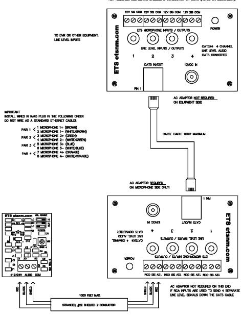
TO ETS BASE STATION MICROPHONE NPUTS, 12V CONNECTIONS NOT REQUIRED, USE 22AWG SHELDED 2 CONDUCTOR OR COAX (RG158 OR EQUIVALENT).
