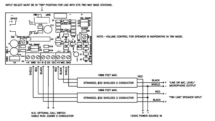
LINE/MIC. LEVEL MICROPHONE OUTPUT AND 70V SPEAKER INPUT
